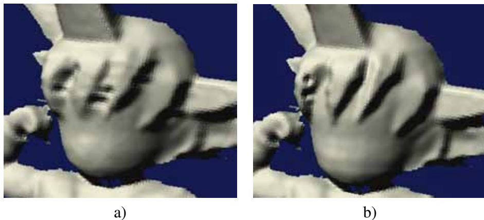
Figure 7.16: Detail of the synthesized depth map : a) Without distortion information, b) Using distortion information
