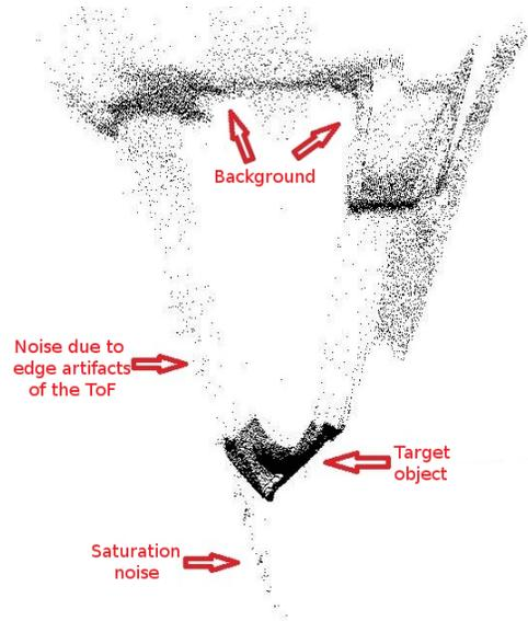
Figure 3. Sample view of the *ball* scene from the experimental results showing some examples of the artifacts in the data acquired by the ToF sensor.
