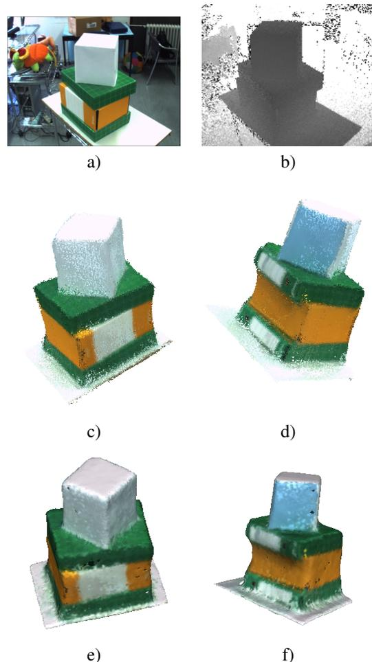
Figure 6. Reconstruction of the *boxes* scene: a) Color view of the scene; b) Depth map representing one view acquired by the ToF sensor (*contrast-stretched for visualization purposes*); c) Snapshot of the obtained point cloud; d) Snapshot of the obtained point cloud from another viewpoint; e) Snapshot of the 3D model obtained by simplifying and triangulating the point cloud; f) Snapshot of the 3D model from another viewpoint.
