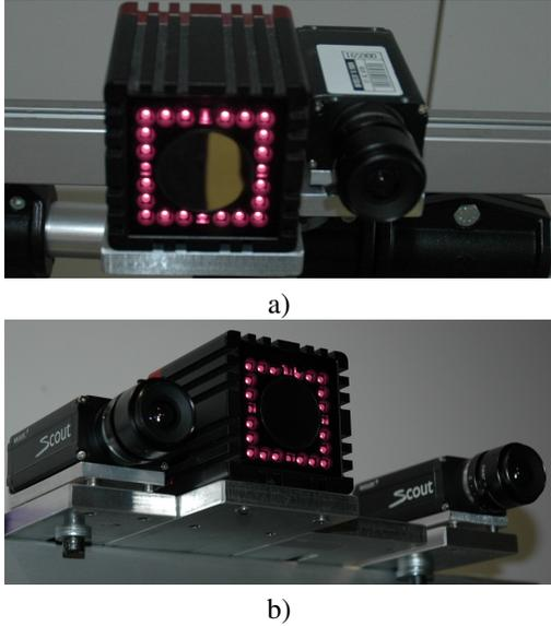
Figure 1. Employed acquisition setup. a) ToF camera and standard color camera; b) extended version with 2 color cameras.
