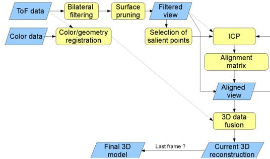
Figure 2. Architecture of the proposed system
