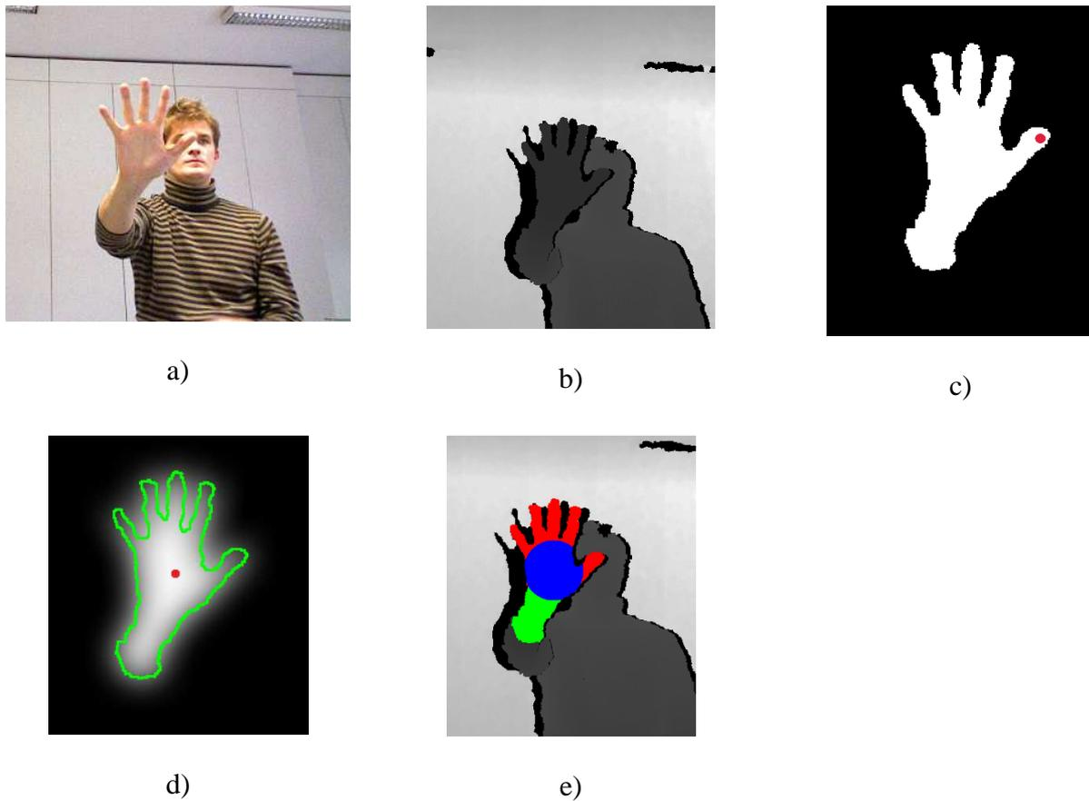
**Figure 2.** Extraction of the hand: a) RGB image; b) acquired depth image; c) computed hand mask (the red point correspond to  $X_{\min}$ ); d) blurred depth mask with C dotted in red; e) segmented hand regions. (best viewed in colors, some images have been cropped to highlight the areas of interest)
