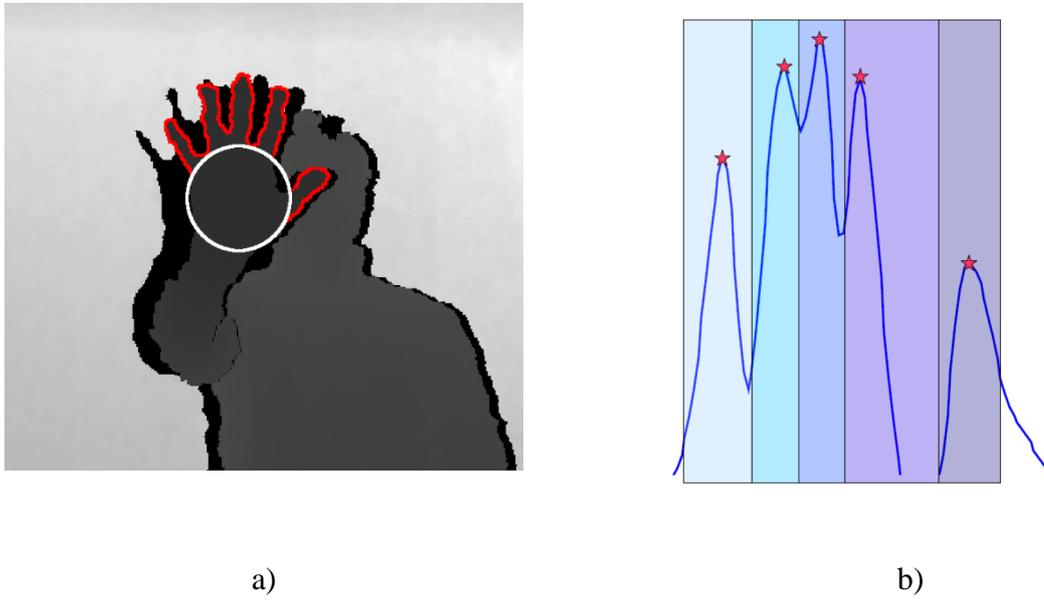
**Figure 4.** Histogram of the 3D distances of the edge samples from  $C$ . The colored areas are the features regions: a) finger edges computed from  $F$  ; b) corresponding histogram  $L(\theta)$  with the regions corresponding to the different features.
