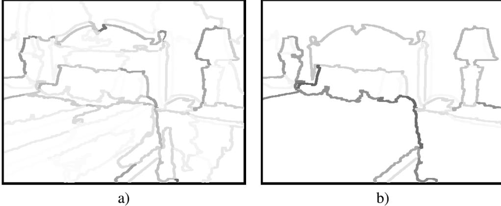
**Fig. 4.** Similarity values  $b_{i,j}$  computed on a sample scene: a)  $b_{i,j}$  values between segments in the initial over-segmentation; b)  $b_{i,j}$  values between segments at the end of the merging procedure. The color of the boundary between any two touching segments is proportional to their similarity score (white corresponds to high  $b_{i,j}$  values and black to low ones)
