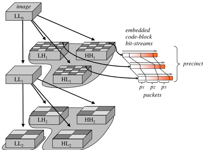
Fig. 8. Basic JPEG2000 elements communicated by JPIP.
