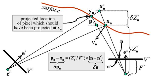
Fig. 5. Relationship between the various coordinates used to map depth uncertainty  $\delta Z_n^*$  at location  $n$  in  $V^*$  into displacement uncertainty  $\delta n$  in  $V^{i \rightarrow *}$ .
