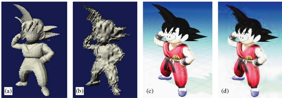
Fig. 18. Some of the Goku view and depth images available at different quality levels: (a) depth map  $Z^1$  at 0.4 bpp; (b) depth map  $Z^1$  at 0.025 bpp; (c) view  $V^2$  at 0.4 bpp; and (d) image  $V^2$  at 0.025 bpp.
