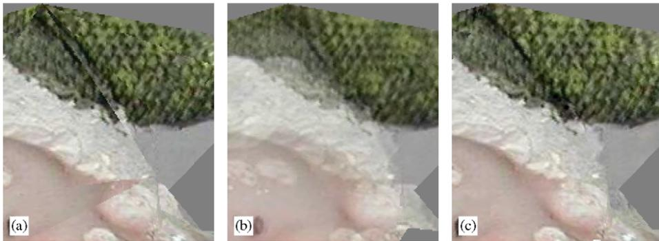
Fig. 13. (a) Image domain stitching; (b) averaging; and (c) multi-resolution stitching.
