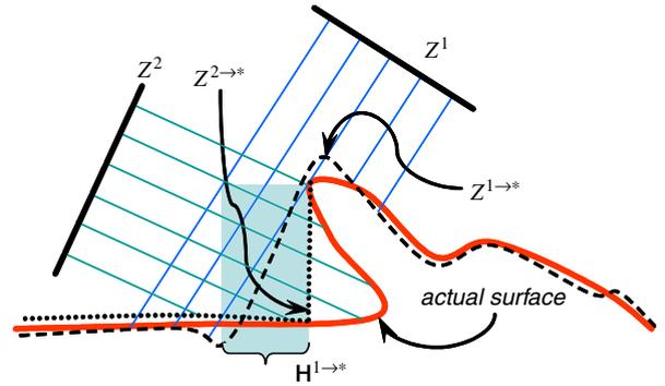
Fig. 7. Illustration of the effect of discontinuities in individual depth maps  $Z^i$  on the synthesized depth candidates  $Z^{i \rightarrow *}$ . In the figure, the depth of interest  $Z^*$  which we wish to synthesize is the vertical height of the surface.
