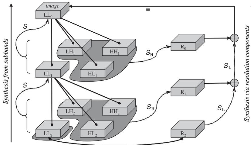
Fig. 3. Relationship between DWT subbands, resolution components and the image which they represent, for the case of a  $D = 2$  level decomposition.
