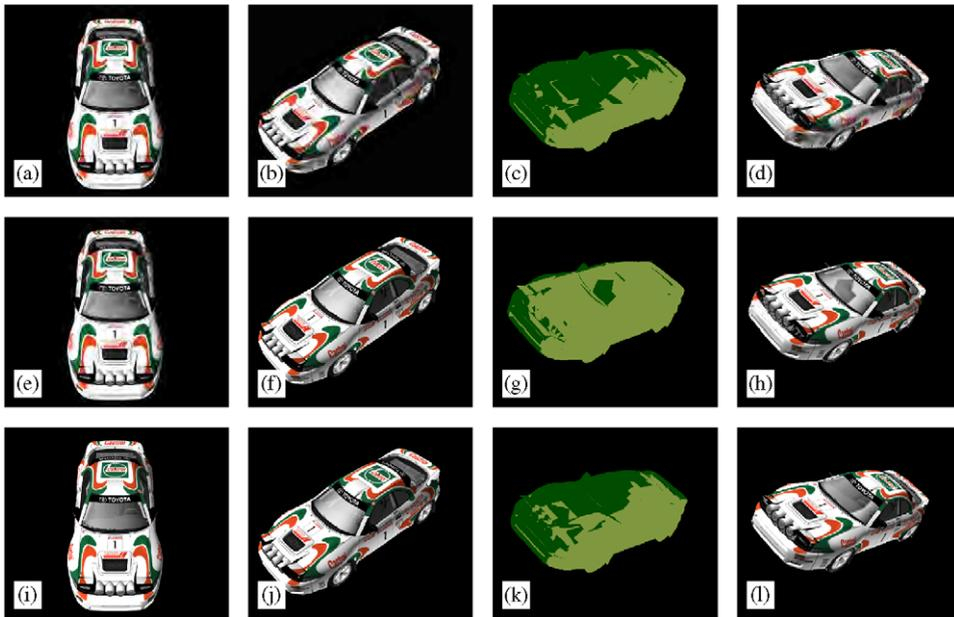
Fig. 17. GT: (a) and (b)  $V^{1'}$  and  $V^{2'}$ , each at 0.025 bpp; (c) and (d) stitching decisions and rendered view based on  $V^{1'}$  and  $V^{2'}$ ; (e) and (f)  $V^{1'}$  and  $V^{2''}$  at 0.025 and 0.4 bpp, respectively; (g) and (h) stitching decisions and rendered view based on  $V^{1'}$  and  $V^{2''}$ ; (i) and (l)  $V^{1''}$  and  $V^{2''}$ , each at 0.4 bpp; (m) stitching decisions and rendered view based on  $V^{1''}$  and  $V^{2''}$ .
