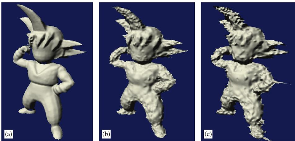
Fig. 19. Synthesized depth map  $Z^*$ : (a) from 0.4 bpp source maps; (b) from 0.05 bpp source maps; and (c) from 0.025 bpp depth maps.
