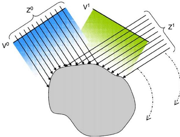
Fig. 6. Browsing environment with a fixed set of views,  $V^i$ , and depth maps  $Z^i$ . In this example,  $V^0$  and  $Z^0$  share the same view point, whereas  $V^1$  and  $Z^1$  do not.
