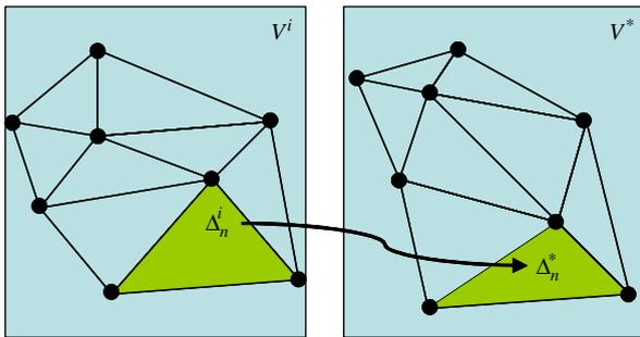
Fig. 2. Surface mesh projected onto  $V^*$  and an original view image  $V^i$ .
