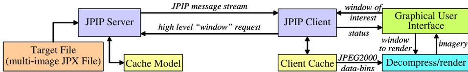
Fig. 9. Client–server interaction in JPIP.
