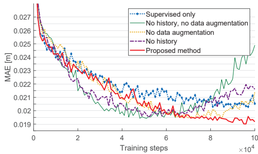
Figure 5: Validation error during the training procedure for different versions of the proposed approach.
